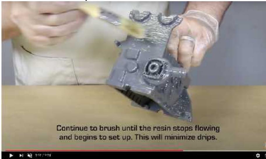
Youtube. Smooth-on. “Smoothing the Surface of a 3D Printed Model Using XTC-3D Coating”. 2014
